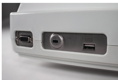
USB and RS-232 interfaces provide speedy communication with computers and printers
